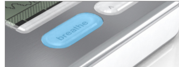
Figure 6. Ambient Feedback: the breathe button under the screen glows to reinforce optimal breathing, allowing the user to stay in a synchronized state without relying on the LCD screen.
